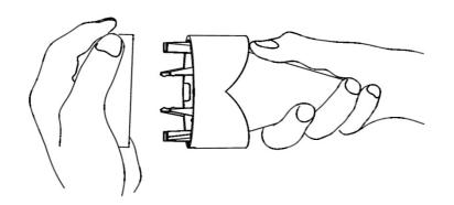
Right Hand gripping the Lens when fitting the lens
