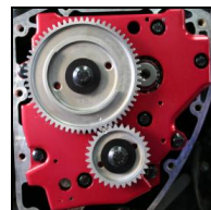
*Gear drive cams mounted on camplate #8000
