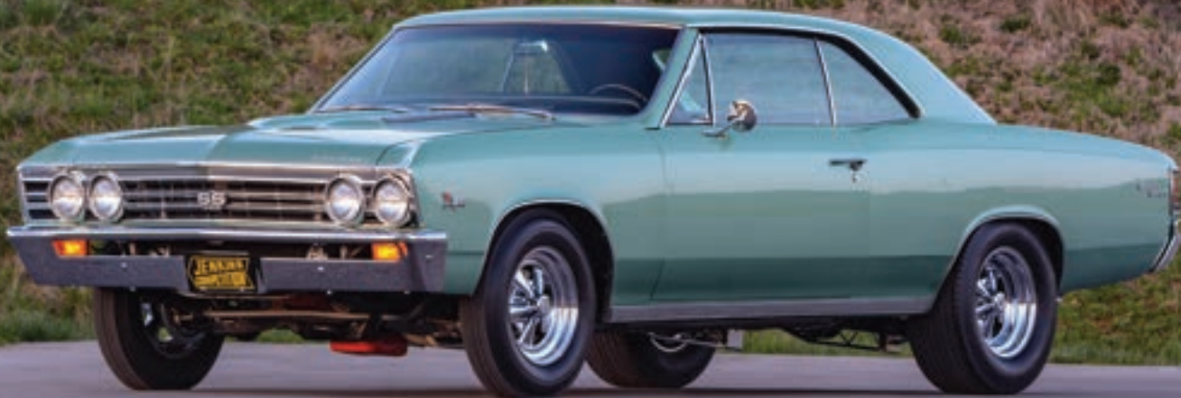
1967 Chevrolet Chevelle SS Wheels: Cragar S/S Front: 15x4.5 Rear: 15x8 Tires: Front: BFG 640-15 Rear: Pro Trac 275/60-15
