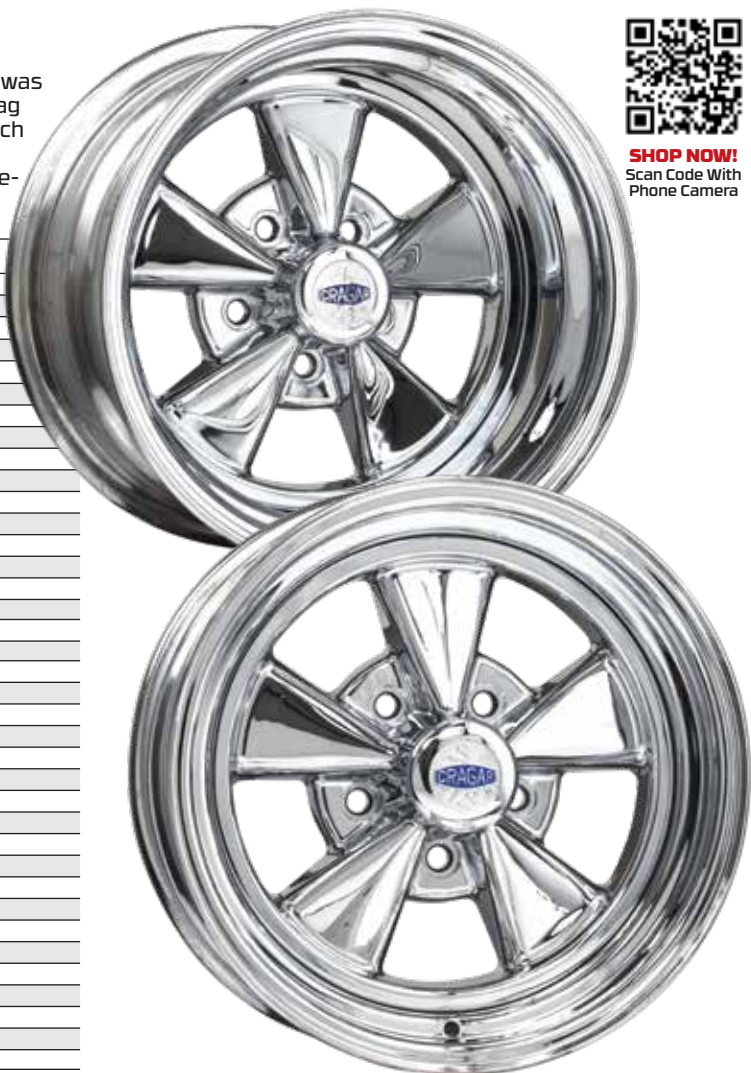
1967 Chevrolet Chevelle SS Wheels: Cragar S/S Front: 15x4.5 Rear: 15x8 Tires: Front: BFG 640-15 Rear: Pro Trac 275/60-15
