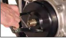
Big Twin Alternator Rotor Puller uses the two threaded holes in rotor to allow removal of rotor.
