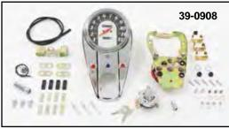
Two or Three Light Dash Kit is complete as illustrated. Includes either 1:1 or 2:1 ratio speedometer and the correct five post key switch with two keys. Order plainbase dash kit when it is not desired to rewire harness for dash lighting. Choose proper cable for each application. Can be mounted on 1947-84 FL Big Twin models.
