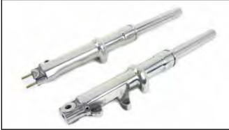
**FXWG Polished Lower Leg and Fork Tube Set h**as 1980-1983 polished lower legs that has no reflector boss and has early style horse shoe type fender mounts. 2 lower legs and 2 fork tubes only. Does not include internals, springs, plugs or lower leg cap. Fits1980-83 FXWG.
