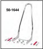
**One Piece Rigid Mount Sissy** Bars features a steel upright that is welded to the rigid mount side plates. Bolts directly to fender struts for a narrow profile and clean installation. Back rest pad is not available. Note: Installation hardware included but the required docking hardware kit must be ordered separately. Fits 2018-up FLDE, FLHC, FLHCS, FLSL, FXBB. 21" is height.
