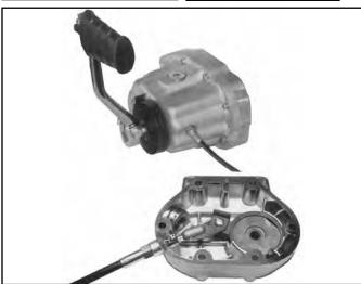
**E-Z Pull Clutch Assist** reduces manual effort required to pull the clutch lever by 40%. Mechanism fits inside transmission side cover and extends clutch operating mechanism for improved leverage.
