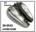
**Bobbed Gas Tanks** fit 1936-84 FLH-FXE with Bobbed tank type mounts for years listed not FXR or FLT models. Tanks accept stock dash and speedometer. Order cap set separately and petcock separately.
