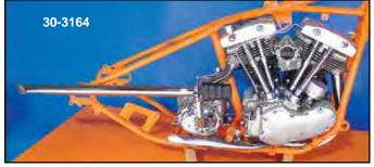
Shot Gun Exhaust Headers fit Rigid frame only. Pipes have 13/4" outside diameter unless noted.
