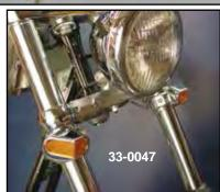
Chrome Fork Mount Turn Marker Bulb Lamp Set is a die cast two piece housing with 12 volt bulb, to attach to 35, 39 and 41 mm fork tubes.
