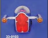
Wide Tombstone Tail Lamp Assembly feature LED units in turn signal lights to fit stock 1973-99 rear tail lamp cutout. VT No. 33-0103
