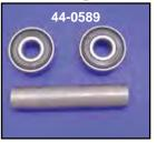
**Deluxe Rear Hub Rebuild** contains all internal parts including longest length inner spacer (white 4.4480). Spacer can be cut down or collar removed for some applications.
