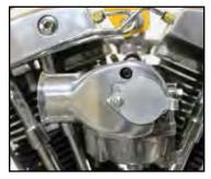
1%" "E" Carburetor Air Intake Snoot Kit constructed of cast aluminum with a polished alloy finish. Includes the carburetor air snoot door.
