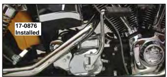
**5-Speed Kick Starter Kit** features slim profile design. Order kick starter arm and pedal separately. Fits all 5-Speed FXST, FLST, FLT and FXD replacement OEM transmissions.
