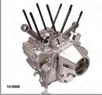
V-Twin™80" Short Blocks are shipped fully assembled as shown. All 80" units feature an S&S Crankcase, Sifton Oil Pump/Breather assembly, stock stroke flywheel, Timken Bearings, stock cam properly installed with a matched pinion and cam gear with Torrington bearing. Assembly is supplied with a chrome nose cone cover and chrome lifter blocks are fitted with standard tappets.
