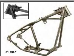
Replica Retro Rigid Frame features original style construction including forged parts in neck, side car mounts and rear axle areas. 103/4" between the rear axle plate. Order rear mount for TC-88 models separately.
