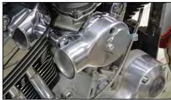
Polished Carburetor Air Intake Snoot with adapter ring to fit CV carburetors. Constructed of cast aluminum with a polished finish for S&S and shorty carburetor applications. Includes the carburetor air snoot door. \*Note: Carburetor will still require a support bracket or breather-bracket combination. Fits 1988-2006 XL and 1993-06 FX. VT No. 34-1403
