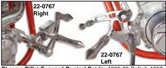
Chrome Billet Forward Control Set fits 1986-99 Softail, 1958-84 FX-FL. Includes rubber belted pegs as shown. Includes shifter side and brake side with master cylinder. Order shifter rod and stainless steel brake lines separately.
