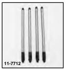
V-Thunder Evo Pushrod Sets are made from .049 wall 4130 chromoly steel. Exacting tolerances for reliability. VT No. 11-7712 is a 2-piece style which can be removed or installed without disassembling heads. These rods fit stock or Velva Touch Tappet units. \*Note: Saves time without the disassembling of the heads or tappet blocks
