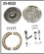
Glide Front Brake Backing Plate Kits consist of all hardware including brake shoes, springs, backing plate, drum, axle sleeve, nuts, cam with lever and mount stud. Available for left side 1949-69 and right side 1969-71. Chrome kit includes chrome drum and chrome backing plate. Black kit includes black drum and polished backing
