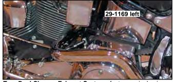
True Dual Chrome Exhaust Systems feature a single pipe for each side. Each pipe is independent and has 13/4" outside diameter. The rear pipe is for the left, and the front pipe is for the right without intersection.
