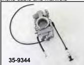
OKO Natural Flat Side Carbs Includes enricher, idle adjustment cables, air cleaner flange mount and air cleaner adapter ring. Uses stock choke cable, manifold and air cleaner. Order manifolds and related parts separately.
