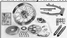
Swingarm/Brake Assembly Kit for 1958-85 FL-FX contains all parts pictured, for stock tire width. Includes chrome swingarm with pivot pin and bearing kit, chrome caliper and bracket, caliper anchor arm, 10" or 11.5" drilled steel (zinc) rotor, 16" x 3" complete chrome wheel, 51T chrome sprocket, 12" FX (spring) or FL covered shock set with shock studs and chrome axle
