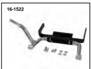
Adjustable Display Center Stands show your bikes. Single lever on left side allows bikes to be lifted up on stand. Very little effort required. Entire assembly fits neatly under frame rails. 2 bolt installation. Caution: Not intended for use as a ride off stand.
