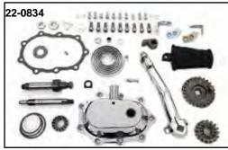
**Heavy Duty Kick Start Kit** features a chrome smooth thick wall kick cover and heavy duty kick starter arm. Fits all 4-Speed Big Twin 1936-84. Requires use of wafer type release bearing kit.
