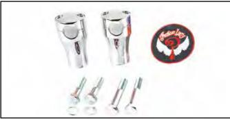
Indian Larry Riser Set features chrome solid billet 3" risers for 1" handlebars with ½" - 13 mounting threads. Handlebar riser bolts are included.
