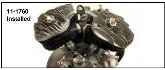
Head Set is for 74" and 80" models. This set is casted after the OE Cast Iron Heads, which feature the squish "WR" combustion chamber. Head set accepts 1 3/8" 18mm spark plugs. Fits 1937-48 UL.
