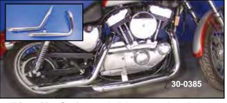
**21/4" Drag Pipe Set** features built in mount tabs to bolt to stock bracket. Chrome replacement bracket and baffle set available separately. Fits 1986-03 XL models.
