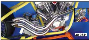
X Series Pipe Sets fit right or left side drive applications.
