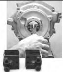
1990-98 Big Twin Snap Ring Remover will remove the Timken Bearing outer race snap ring without damage to the case.
