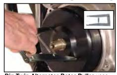
**Big Twin Alternator Rotor Puller** uses the two threaded holes in rotor to allow removal of rotor.
