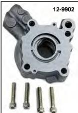
**Twin Cam Super Pump** by Sifton utilizes an oversized highly efficient Geo Rotor design. Provides a 40% increase in pump volume and a 60% more scavenging volume. This high volume pump bolts into the stock location and includes O-Rings and mounting hardware.
