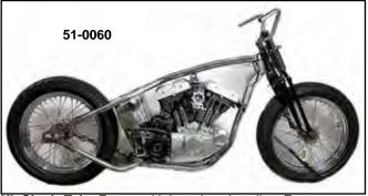
XL Single Tube Frame with board track styling. Features a distinctive 13/8" diameter, single loop front downtube and 11/8"diameter lower frame rails. The rake is set up to use stock length replica Springer Forks with 1" stem. Engine mounts are cast steel for strength and aesthetics! Single loop frame is constructed to give the look and feel of an early board track racer. Fits 1982-03 XL.
