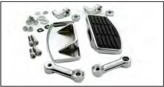
Adjustable Driver's Mini-Footboard Kit measures  $7\frac{1}{4}$ " x  $3\frac{1}{2}$ " male end. Fits into stock female footpeg clevis on models with forward controls and features  $\frac{7}{8}$ " of fore-to-aft movement, they may be rotated in a  $360^{\circ}$  arc.
