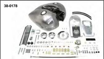
**Bobbed Tank Kit** for 1995-05 FXD models are 4 gallon available with chrome cast dash assemblies which include a Bob type 6 post key switch and a plain dash base. Pre 1995 units include a Bob speedometer. 38-0178 kits include an adapter ring to allow reuse of the existing electronic speedometer. Chrome caps included.
