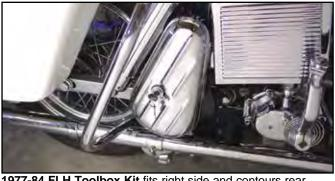
1977-84 FLH Toolbox Kit fits right side and contours rear shock and bolts to rear battery tray and exhaust tube mount. Kit allows use of FXE or FLH exhaust.
