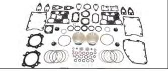
Wiseco Twin Cam Big Bore Piston Kit for 2007-17 Twin Cam 96"/103" bored to 1802cc (110 cu. in.) X-ring package (10.5:1 comp. flat top) also fits 99-06 Twin Cam 88 with 4%" stroker crank. Kit includes top end gasket set. VT No. 11-0849
