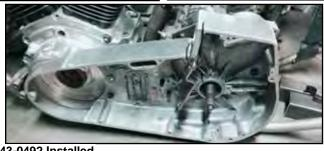
43-0492 Installed FXE-FLH Inner Primary Cover Assembly for 4-Speed models.
