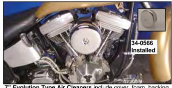
**7" Evolution Type Air Cleaners** include cover, foam, backing plate. Order brackets separately.
