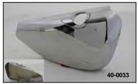
Chrome Oil Tank Covers are of one piece form fitting design to fully cover the outer surface of the tank. Cover is easily installed without removal of tank. It is attached to the rear oil tank fittings by springs supplied on 1983-93 model and by clips on 1994-up models. Chrome except where noted.
