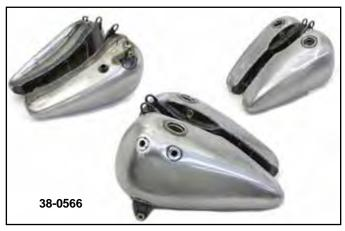
Fat Bob 3.5 Flatside Bobbed Tank Set features handshift gate provisions to fit early style gates for 1936-46. These flat side tanks feature screw type bungs. Order caps separately. Petcock fitting should be masked or plugged during painting for easy installation. The side tank features side shift tank mounts. For use with cateye 1936-1946 type shifter gates or the conversion gate for 5 and 6 speed models, smooth type.
