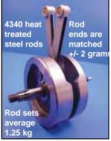
**Flywheel Assemblies** feature full weight flywheels, with removable pinion and sprocket shafts as original, trued and balanced for cast pistons. Units include forged and machined H-Beam Sifton connecting rod set of certified 4340 steel with multistage heat treatment and are fitted with Torrington Rollers, with alloy bearing retainer cages.
