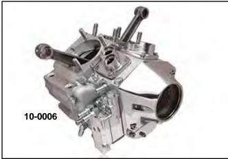
V-Twin™80"Short Blocks are shipped fully assembled as shown. All 80" units feature an S&S Crankcase, Sifton Oil Pump/Breather assembly, stock stroke flywheel, Timken Bearings, stock cam properly installed with a matched pinion and cam gear with Torrington bearing. Assembly is supplied with a chrome nose cone cover and chrome lifter blocks are fitted with standard tappets. Blocks fit 1973-84 Shovelheads.
