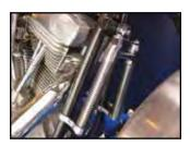
Chrome Billet V-Cooler will mount to front frame tubes as shown. Unit is 41/8" wide at the top. Each tube 10.5" long and 11/8" in diameter.
