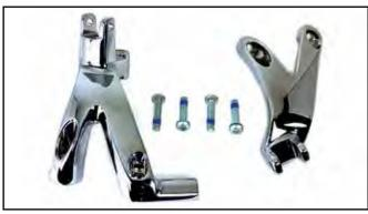
Chrome Standard Forward Control Mount Kit replaces the factory painted forward control mounts. Fits 2018-up FLSB, FX. VT No. 27-0180
