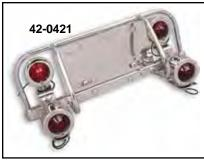
Chrome Dresser Lamp Bar with four bullet lights and license plate backing plate. Mounts on stock FLH or FLT license plate bracket. For 71/4" x 8" license plate. Fits 1958-84 FLH.
