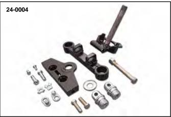
**Black Adjustable Fork Tree Kit** is available for 1977-84 FLH, FXWG 41mm fork legs. Showa type is 1977-up. Kits feature swivel type plugs which are included. Lower tree has two positions for changing rake and fork lock tab. Kits use VT No. 28-0221 rubber bushing kit and VT No. 24-9910 top tree cover.
