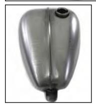
Chopper Axed 3.3 Gallon Gas Tank Gas has a right side petcock opening, and a fuel capacity of 3.3 gallons. Features a bayonet type bung. The tank features center rails and two mount tabs, and a %" NPT outlet with 2 x ½" cross over outlets on either side of the rear to allow for multiple choices for routing fuel lines. VT No. 38-0680
