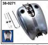
2" Stretch Tanks fit FXDWG models with stock dash. Tanks accept right and left side bung cap set.
