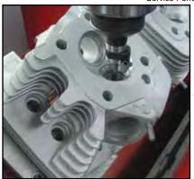
Motor Shop Ready Head Remanufacturing Service. Available as a valve job only or as a valve seat/valve job remanufacturing service. We will glass bead heads, install new cast iron guides, nitrated coated valves, spring, collars and keepers for both services. For valve seat
