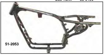
Swingarm Frame will accept 1983-90 oil tank, gas tank, 1994up battery carrier, 1982-93 rear fender, struts and 1" Big Twin chrome neck cups. For belt or chain drive.
