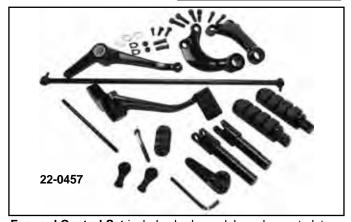
**Forward Control Set** includes brake pedals and mount plates as shown.
