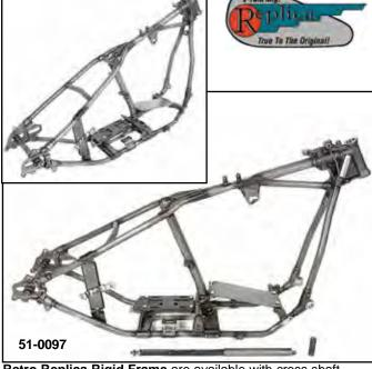
Retro Replica Rigid Frame are available with cross shaft tube to accept stock mechanical brakes and star hub wheel. Replica retro rigid frame original style is updated to accept flat side tanks. Original forged parts include: neck, side car mounts and rear axle area plates. For all Big Twin engines with 4, 5 or 6 speed transmission. Features +2" raised neck and 10.75" between the axle plates. Will fit mechanical brake drum assembly with a 140 tire.
