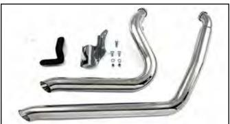
Chrome 2" Side Sweeper Exhaust Pipes fit 5 and 6-Speed 1986-17 FXST models without footboards. Pipes have 18mm oxygen sensor bungs and includes plugs for non EFI applications which can be removed for 2007-17 models to install sensors.
