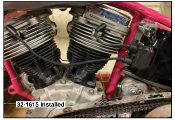
Coil Mount with key switch bracket.
