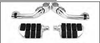
Highway Bar Kits clamp on 11/4" diameter tubes.
