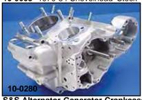
S&S Alternator-Generator Crankcase Set is shipped with left side bearing race, oil pump drive bushing, cylinder base studs, idler stud, circuit breaker stud, pinion needle bearing and pinion race installed. Pinion race is lined. Honed and ready for assembly. Also included are nickel plated case bolts, crankcase fittings, left side engine bearing, seal and spacer. Accepts wheels up to 81/2" diameter.
