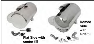
Round Oil Tanks fit 2000-17 Twin Cam-Softail models with side fill. Tank is 6.5" diameter, 11.75" long and requires removal of coil bracket and relocation of coil. Order mount kit separately. Note: Will not fit rocker models.
