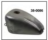
**'King' Gas Tanks** are made 2" wider than stock and include stock style mounts, 3.1 gallon capacity and uses 1975-up type petcock on 1979-94 type tanks. King Tank is 17½" long, 10¾" wide. Petcock side as noted.
