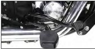
**2" Forward Mid Control Kits.** Comfortable as slightly more forward than stock 2006-17 FXD mid controls. Stock replacement for 2014-17 FXDL.
