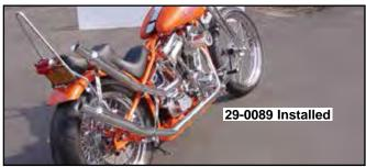
Chrome 1¾" Up Sweep Header Sets for 1986-06 FXST models. Use with straight fishtail extensions or mufflers which must be purchased and mounted separately. 1986-99 applications will also require separate purchase of correct mounting brackets.
