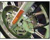
2000-07 Front Caliper are 4 piston type including all internal components. 23-0554 features smooth face.
