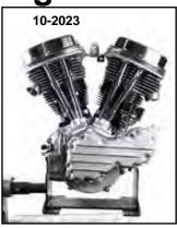
Replica Panhead 74" Engines have replica type heads with stock exhaust ports and V-Twin cases. The 1948-54 style uses a plumber intake manifold. The 1955-61 style uses O-ring intake manifold. Engines include cast iron oil pump. OE number boss in provided blank on left side. Actual case numbers are on right side. The sprocket shaft supplied is for 1936-64 style 4-speed stock transmissions. Engines listed do not include intake manifold.
