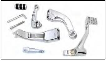
2004-05 XL Stock Mid Control Kit is for use with stock footrests. \*Note: Order additional hardware and reuse original components from the motorcycle.
