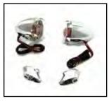
Rear LED Bullet Style Turn Signal Kit. The red wire is the running light, the black wire is the ground and the black and white wire is the turn signal.
