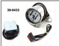
Multi-Colored 60mm Speedometer. The gauge features a 2.4" polished stainless body and a white face, a total length of 2.7". Units include a chrome bezel with choice of red, orange, blue, yellow, white, green or purple by the push of a button, works on a 12 volt system. Tachometer adapter required for use with single fire ignition. Speedometer accepts 12 mm drive cable. Order clamp separately.
