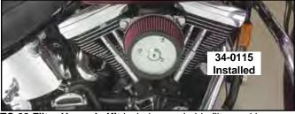
TC-88 Filter Upgrade Kit includes washable filter and longer stud set to replace Screamin' Eagle elements. There is 20% more air flow with this filter. Order cover separately.
