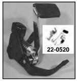
2000-06 Brake/Shifter Side Components for TC-88 models FLST, FLSTF, FLSTS. FLST style controls accept footboards.
