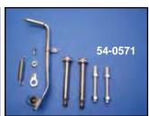
"Full" Lowering Kits include components to lower the front and rear of Softail models. Each kit includes shorter damper rods, 1" shorter kickstand and adjustable rear shock lowering set. The front of the FXST is lowered 2.5" and 2" on FLST models. Rear is adjustable up to 1.5" on 2000-06 models and up to 2" lower on 1989-99 models, using stock shocks.
