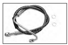
**10mm Stainless Steel Banjo End Dual Disc Upper Hose** fits 1982-up style master cylinders for single or dual disc application. Hose has nut with inverted flare at opposite end. The length from the banjo to the first bend is 24".
