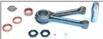
**S&S Rods** are replacement rod sets included wrist pin bushings, rod races, matched rods, pins, rollers-cages, and nuts, for stock or stroker use. Use "Supreme" which is recommended for drag strip applications. Fits 1981-85 XL.
