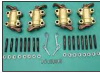
Rocker Arm Assembly includes all pieces to completely assemble the rocker arms on both heads. Includes four rocker housings with matching fitted rocker arms, heat treated studs tubes and dowel pins.
