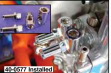
**Chrome Tight Spot Oil Pump** Fitting Set features a 5/16" allen socket for easy installation or removal. Includes 1/8" NPT nipples. VT No. 40-0577
