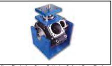
Jims Evolution Case Cylinder Spigot Bore Tool allows boring of cylinder spigot hole, up to 3.8125" by utilizing the stock cylinder stud holes. Use on all 1984-99 style Evolution crankcases
