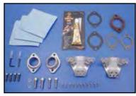
Tru Seal Manifold has two machined manifold halves which bolt together with stainless allen screws. Does not require the use of existing stock style O-rings or seals. Evolution type includes front and rear head spigots, gaskets, sealing compound and instructions included. Fits 1985-98
