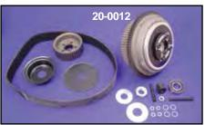
Brute III from Primo Products includes dry clutch pack pulley assembly which retains diaphragm spring function, while increasing the clutch friction surface area 70% for smooth light fingered action. Kit includes pulleys, 1¾" Kevlar reinforced rubber belt, complete clutch pack/pressure plate assembly and necessary hardware, bolt in kit. Available in 8 mm or 11 mm drive kits.
