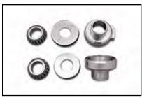
features built in fork stop on lower cup to accept 1988-99 FXST lower fork stem with integral stop. Kit includes chrome upper and lower cups with races, bearings and dust shields.
