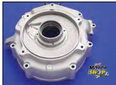
**Motor Shop Alternator Sealing Ring** Replacement Service. Ship in 1970-up left VT No. 16-0693 hand case with damaged O-Ring lip and we will machine out and replace with new steel sealing ring.
