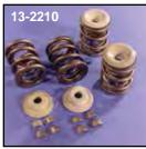
Kibblewhite Lightweight Valve Spring Kits include springs, keepers, retainer, and lower collars unless noted. Fits 1970-84 XL for 160 lb seat pressure, up to .460" valve travel. Hard-anodized aluminum retainers. May require "R" model valve to achieve installed height.
