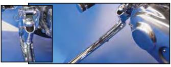
**Custom Kickstand Assembly** features full forged construction with chrome smooth contour design, including recessed mount screws for 1936-99 Big Twin, 4-Speed, 1984-up Softail models. Stock length.
