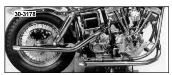
30-3178 with over the transmission rear pipe fits kick start only in Rigid or Swingarm frame
