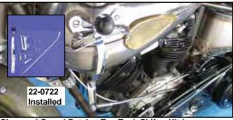
Chrome 4 Speed Ratchet Top Tank Shifter Kit features smooth gate, handle and rod and pivot bolt for 3.5 gallon tanks for years listed.
