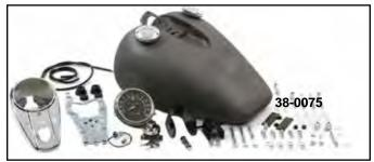
Bobbed 3.2 Gallon Gas Tank Kit for 1952-78 XL. Gas tank is dual cap style with a left side petcock location, and a fuel capacity of 3.2 gallons. Kit has a one piece tank that will bolt to existing mounting holes. Includes three light dash cover kit, bobbed tank mount bracket, chrome gas cap set, and front bobbed dash speedometer cable, and 2:1 speedometer.
