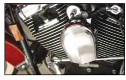
Chrome Head and Spark Plug Cover fits 1986-99 Evo models. Covers are held in place by rubber inserts supplied.
