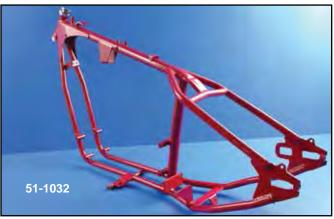
Rigid Frames for XL models will accept 1" neck cups, VT No. 24-0119 and include mounts for flat side fat bob tanks or stock tank. Frames with cross shafts include bushings. Order oil tank and battery box separately. Disc brake models accept 1987-99 caliper assembly VT No. 22-0370 and a 140 tire. All frames have 40° rake and 1" stretch. 1975-76 models require use of forward controls. Note: 1957-79 application requires modification of rear motor mount to accept kick shaft.
