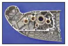
Motor Shop Cam Cover Bushing Service will install new bushings in cam cover for 1957-up XL models. VT No. 60-0131
