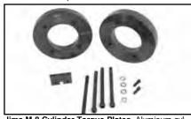
Jims M-8 Cylinder Torque Plates. Aluminum cylinders cannot be accurately honed and measured without the use of torque plates. The Jims Torque Plate kit for use on Milwaukee-Eight ® cylinders will simulate operating stress conditions when boring or honing cylinders. These plates adapt easily to conventional boring bars or Sunnen honing machine, and do not require the removal of ring dowels. Use on 2017-up Milwaukee Eight® engine
