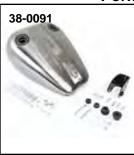
Porkster Tanks feature a smooth top and does not accept dash panel or speedo. 3.2 gallon capacity and includes necessary hardware for installation. Order cap set VT No. 38-0321 late bung style caps separately.1995-up kits include coil/ignition switch kit. Tank width is 141/2" tapering to 9", overall length is 19", tunnel height is 71/2" and width is 21/2".
