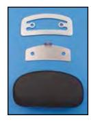
Flatlander Mini Back Rest in black features a stainless steel insert with chrome frame mounting system for short sissy bars. Measures 5½" wide x 1¾" tall x 2½" thick.
