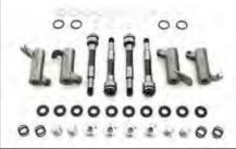
Sifton Rocker Arm and Shaft Kit fits 1957-84 XL Iron Head models and includes four rocker arms with bushings installed, four shafts, shims, spacers, chrome replica end caps and nuts.
