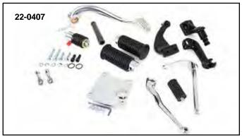
FXR Mid Control Kit includes the shifter and brake pedal.
