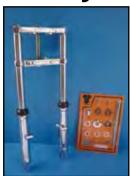
FXST Style Single Disc Fork Assembly features chrome trees with 1" stem, polished or chromed lower slider legs, to accept 11.5" caliper and brake disc, hard chrome fork tubes, axle, neck bearings, top cone and stem nut, pinch bolts and bearing dust covers. Fork is 31" overall length (L) and legs are assembled. Single disc unit accepts 11.5" brake disc and left side caliper.
