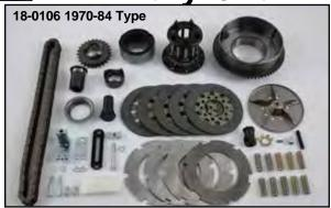
Primary Chain Drive Systems for Big Twins include 76 or 82 link primary chain, chain shoe adjuster assembly, clutch drum basket with starter ring gear and steel and fiber clutch plates with pressure plate assembly. Correct front compensator sprocket assembly includes all parts necessary for installation, including sprocket nut. Big Twin 5 Speed Softail models and all pre1985 FLH-FX 4-Speeds require 82 link primary chains; 1980-up FLT-FXR 5-Speeds require 76 link primary chains.
