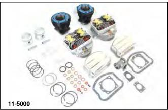
**Panhead Big Bore Kit** with cylinders and matching complete Panhead heads. This kit will fit Panheads-Shovelheads to convert to Panhead type, with overhead oiler system.
