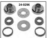
**Chrome Internal Fork** Stop Kit includes pieces for complete installation on Big Twins, and custom frames which accept press in neck cups. Kit allows choice of turning radius of 35 or 45 degrees. For 1936-87 Big Twin in 35° and 45° config-
