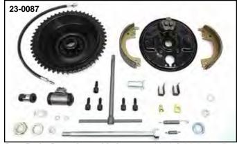
Rear Brake Drum Assembly features a black finish hydraulic drum and backing plate and a parkerized axle kit. \*Note: Shoes are wide type. Fits 1971-72 FX and 1967-72 FL. VT No. 23-0087
