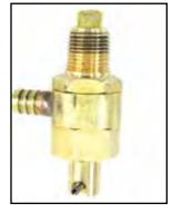
Trock "TRO CY" Brass Petcock features "full bore" flow. Solid machined natural brass, with 3/8" NPT thread and 3/8" hose end. VT No. 35-1955
