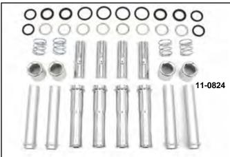
Performance Pushrod Sets for Twin Cam are E-Z install type which are designed to be installed without removal of the heads or rocker boxes. Rods feature chromoly tube construction with rolled thread adjusters. Fits 1999-17 FXST-FLST-FXD and 1999-16 FLT.
