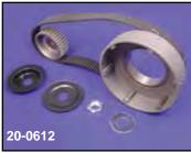
BDL 8mm Belt Drive available in 1½", 2" and 3" for all 1936-84 Big Twins with 4-Speed Transmission with Kick start on electric start. Can be used with stock type clutch or BDL Competitor Clutch. All 2" and 3" Belt Drives include Big Fix Bearing Kit.
