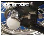
**Chrome Rear Axle Caps fit** 1987-06 FXST-FLST models, completely covers axle ends and cotter key area. Easy to install.
