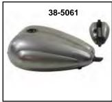
Saga "Dish Gas Tank" is 3 gallon and features dished sides. VT No. Cap
