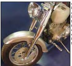
41 mm Fat Kid Style Fork Assemblies Only. Include chrome top tree, black lower tree with polished or chrome lower sliders assembled with hard chrome fork tubes and axle kit.
