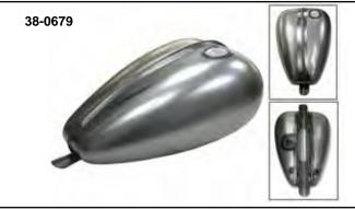
Screw Center Ribbed Axed Tank is a chopper axed gas tank. It has a right side petcock opening, and fuel capacity of 3.3 gallons. The tank features a screw type bung. The tank features center rails and two mount tabs, and a 3/8" NPT outlet with 2 x 1/4" cross over outlets on either side of the rear to allow for multiple choices for routing fuel lines.
