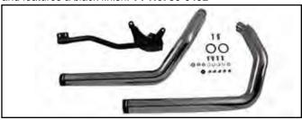
Chrome Straight Drag Exhaust Set with a unique header design has removable performance baffles and polished black anodized billet aluminum end caps. Fits 2004-06 XL.
