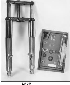
Glide Fork Assemblies feature black lower triple tree without lock tab and accept a left or right side drum brake assembly with chrome or polished slider.
