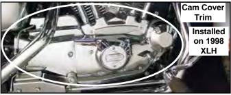
Form Fitting Chrome Steel Covers fit over stock cam cases on XL models. No need to remove cam case or disturb cams or gears. Covers held in place by existing screws and related hardware as supplied. Note: 42-9962 is kickstart only. All other numbers are for electric start.
