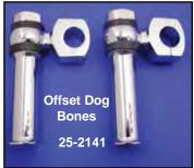
Offset Dog Bones are risers machined of solid steel and chromed includes rubber grommets in riser top vibration damper.
