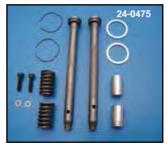
**Fork Damper Tube Kit** includes for 2 sides, damper tubes with rings, screws and washers, lower stops, slider seal washers and retaining rings.
