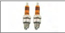
V-Twin Performance Spark Plugs features a copper core electrode for a longer service life, nickel plated housing, 95% pure alumina insulator and a heat crimping process to ensure a leak free seal.
