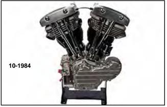
Panhead or Shovelhead 88" Generator-Alternator Long Block features alternator left hand case and generator right hand case. Each long block is assembled with S&S Crankcases, Sifton Oil Pump/Breather Assembly and 41/4" stroke flywheels. See www.vtwinmfg.com for more info.
