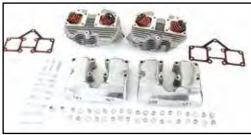
**Cylinder Head Set** with polished rocker box set is assembled with cast iron guides, valve stem seals, and nitrated valves. Heads have complete valve job for maximum flow, horsepower, and torque. Heads are single plug and are assembled with polished rocker boxes. Max lift .450. Sold as a pair.
