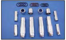
Chrome Billet Pushrod Cover Set for Twin Cam engines and includes seals and O-Rings necessary. Replaces 18096-00. Fits 1999-17 FXST, FLST, FXD and 1999- Replica Pushrod Cover Kit for Twin Cam 2016 FLT.
