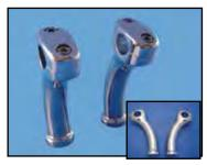
Chrome "Fatty" Curved Riser Set features pull back styling as on 2000-up models. Kit includes two piece cap set and risers with 5" rise and 2" pull back and ½" x 13 internal threads. Replaces 56033-00.
