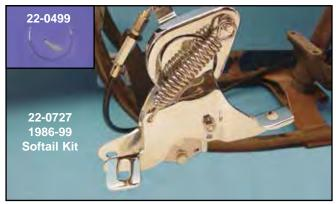
Note: Clutch is disengaged in heel down position.
