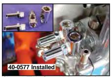
**Chrome Tight Spot Oil Pump Fitting** Set features a 5/16" allen socket for easy installation or removal. Includes 1/8" NPT nipples.
