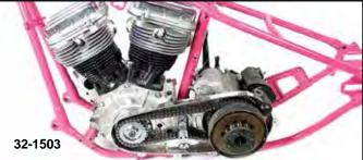
York Electric Starter Kit is complete installation kit. Fits 1941-57 Pan and Knuckleheads. Rear fender and outer primary covers require cutting for installation of kit. 12V charging system, coil, battery regulator and lighting is required but not included kit.
