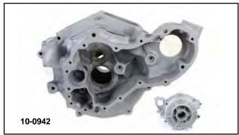
**Knucklehead Case Set** features steel bearing insert cast in. Left hand case available separately is machined to fit OE right side case. Order cylinder base studs and case race separately. **Note:** Cylinder deck height must be finished to match your case.
