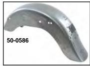
Replica FLST Replacement Rear Fenders. Can also be used on all 1986-up Softail models uses 33-0301 tail lamp and includes indent for turn signal bar.
