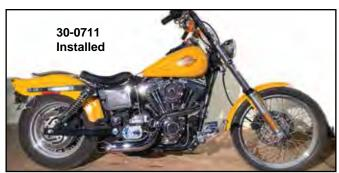
2:1 Lake Side Pipe Exhaust Kit with a turn out end. Available in chrome or black finish and includes heat shields. Features a 3" collector with turn out end. Collector has no baffle. Exhaust Pipe is 13/4" diameter at cylinder head and 2" diameter before collector. Pipes have 18mm O<sup>2</sup> sensors. Fit 1991-17. \*Note: 2012-17 will require 32-6578 O2 sensor reducers.
