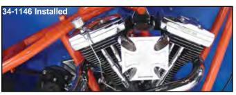
**Chrome Maltese Carburetor Cover** includes backing plate and filter. Kits include brackets and or breather kits as required to fit stock original carburetor. Center portion of cross is matte chrome finish.
