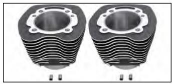
M-8 Big Bore Black Cylinder Set with machined edge fins increase the bore size from 124" to 128". These cylinders have 4.250 bore and require the use of Wiseco piston set 11-9983. For use with stock 4.375" flywheels but require case boring. Black cylinder set with machined edge fins also feature a slightly larger fin area for better heat dissipation and increased
