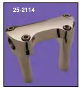
**41/4" Straight Riser Kit.** Stems replace 56142-80 as stock on all 1980-up FXWG. Complete, with riser cap and screws. Use 1/2" x 13 mounting bolts.
