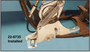
**Note:** Clutch is disengaged in heel down position.
