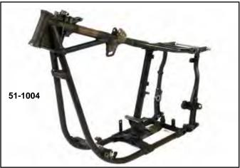
V-Twin Swingarm Frames are our authentic reproductions of FLH styles for the years listed to accept Panhead or Shovelhead engines, 4 Speed Transmissions, seat posts and round or square swing arms. Details include forged parts as original in neck, engine mounts, front transmission mount, top seat post yoke, strut and swingarm pivot mount and footboard mounts, as required. All stamped components are pressed and formed as stock.
