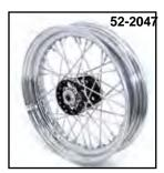
**1936-66 Big Twin Star Hub Type Wheel** includes chrome hub, chrome rim and choice of chrome or stainless spokes. Fits front or rear and hub and is assembled like stock with loose type roller bearings. All wheels include rubber rim strip installed.
