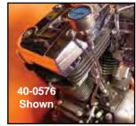
Rocker Box Mounted Oil Gauge Kit fits 1984-99 1340 Evolution Big Twin models. Kit includes a complete liquid filled gauge, chrome steel line and hardware for installation. Kit is available with lower fitting allowing stock oil pressure sender unit to be retained in conjunction with oil pressure gauge.
