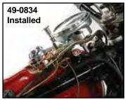
Linkert Choke Cable Assembly includes cable, knob and cable bracket, carb arm for carburetor and hardware. Fits cateye, two and three lite dash panels. Order 35-1065 choke shaft for OHV application.
