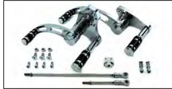
**Chrome Billet Forward Control Kit** includes shift and brake side controls. Kit is stock length with rods included. Fits 1987-99 FXST.
