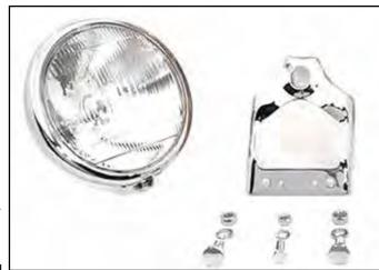
Chrome Springer Headlamp Kit includes chrome 12V Spring Fork head lamp and replica chrome bracket with mount bolts. VT No. 33-1493
