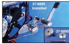
Chrome Brake Lever Pivot Cover Kit fits 1984-99 FXST-FXWG. Includes cover, retainer washer and allen screw. Details this drab area.
