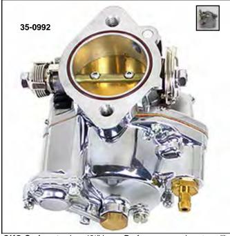
**OKO Carburetor** has 17/8" bore. Performance carburetor will accept S&S jets, and S&S bolt pattern air filter assemblies. This shorty carburetor has a relocated accelerator pump nozzle for increased throttle response, and thunder jets bolt on type.
