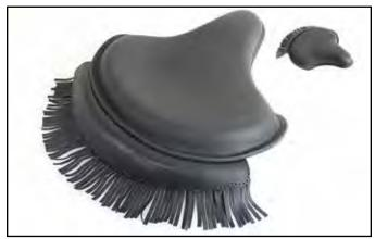
Replica Black Solo Seat has a leather fringe skirt which is tapered from <sup>3</sup>/<sub>4</sub>" to 2" in length. Seat has a molded foam pad on a steel formed and ribbed baseplate with brackets riveted in place. Seams are accomplished by first riveting a leather strip to the seat pan and then formed fitting the leather cover to the saddle and sewing the cover to the strip. It accepts a stock type "T" bar mounting system. Order mount hardware kit separately.
