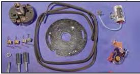
Blue Streak Sifton "Tuneable" Ignition Advance Assembly includes stainless advance base, points plate with "Blue Streak" points and condenser with hardware and 3 pairs of color coated springs which allow full advance at 1400, 2000 and 2600 RPM depending on which spring is selected.
