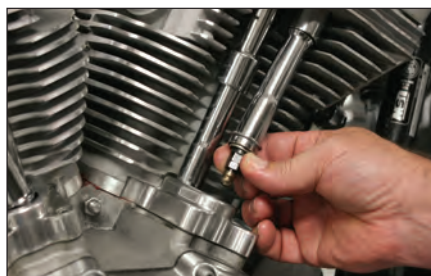
When a Quickee adjustable pushrod is collapsed, it can easily be installed or removed from an assembled engine.
