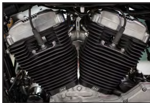
S&S cylinders match the fin profile on 1986–'03 cylinder heads. Although there is a slight difference in the fin profiles of S&S cylinders and stock 2004–'18 cylinder heads (shown above), the look is generally not considered to be objectionable. You decide!
