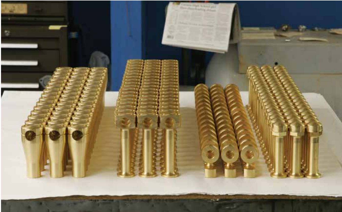
MACHINED SOLID BRASS RISERS READY TO GO TO THE POLISHING SHOP
