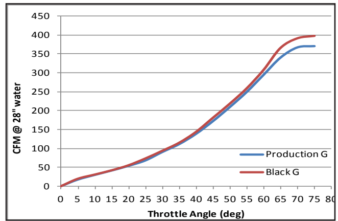
Flow at WOT (wide open throttle) for the Black G carb increases 7% vs. the base S&S G carb
