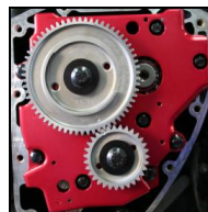
*Gear drive cams mounted on camplate #8000
