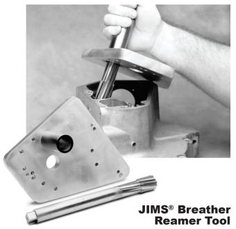
Repair a damaged breather hole without need to disassemble the cases. Using JIMS® Reamer Tool will ream a damaged breather hole to use a .030" oversize breather gear in less than an hours time. For '36-'99 single-cam BT. #758-706
