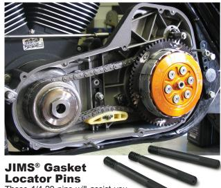
These 1/4-20 pins will assist you in aligning the gaskets during assembly to avoid misalignment and oil leaks. Primary cover, cam cover, and transmission end cover gaskets are just a few of the possible applications. 3 piece set. #758-968
