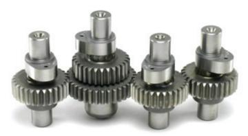
**785V2:** Offset tappet design - the original design of the venerable XL Pro-Stock-Top Gas Cams. This same profile has been used in many championship forms of racing. Net tappet lift is .485"; .785"@ valve with 1.62 rocker ratio. Increase rocker ratio for more valve lift.
