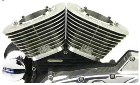
**Zip Tip** ► 3-13/16" is the largest bore size that the stock H-D<sup>®</sup> XL cases can be safely bored for. 3-5/8" bore is the maximum S&S replacement XL/Buell cases can be bored for.
