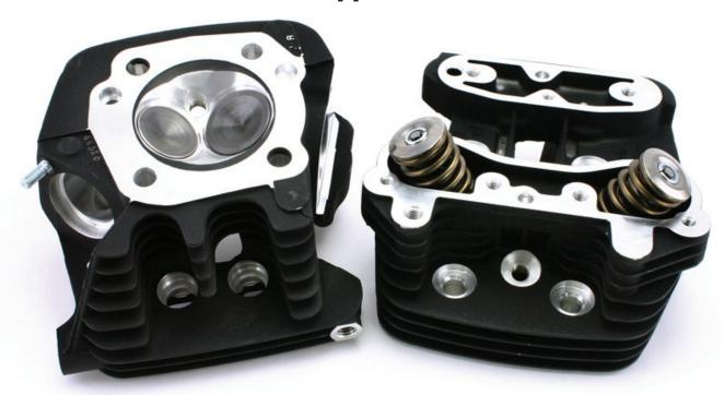
Buell<sup>®</sup> Thunderstorm<sup>®</sup> heads are a popular upgrade for '91-'03 Sportster<sup>®</sup> engines – and they reach Hurricane status with Zipper's CNC port work! After the ports receive the full CNC treatment, Step-Lock valve guides are installed and honed for a perfect fit; the seats are machined to accept larger Baisley stainless steel valves (1.840" intake, 1.615" exhaust) on our
