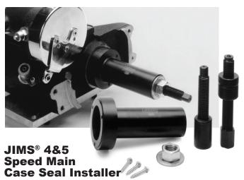
This tool will push the main drive case seal in as flat and straight as possible to .050" below housing for a no leak fit. Tool #758-642 includes the main tool components required and the seal installer for '41-'79 4-speeds. Order drivers for other year 4&5 speed transmissions separately.
