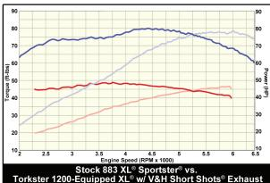
The Torkster 883-1200 conversion is a fantastic value in the power-per-dollar department, as it adds nearly 65% more power to the 883! The Torkster is not just a bore job to increase displacement, but a highly refined cylinder, head and engine management package that promotes big gains in power and torque.
