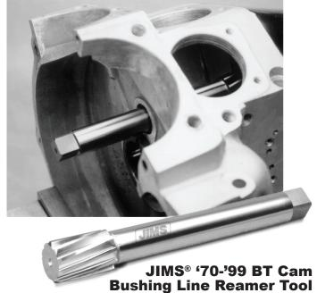
Use to line ream cam cover bushing to size from inner cam bearing on an unassembled '70-'99 single-cam engine. Finish size will be about .0008"-.0015" over the cam journal. #758-845
