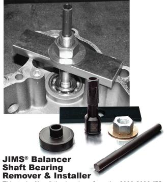
This tool will pull the bearings from the 2000-2006 "B" motor case in one easy smooth motion preventing any damage to the bearing bores. The installing portion of this tool is designed to be used with JIMS® #758-416 tool driver handle to push on the outer diameter of bearings preventing any damage to the bearing or its bore. #758-167
