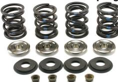
This valve spring kit is designed for use in Shovel or Pan engines with cam lifts of .500"-.580". It is a double spring kit with high strength titanium top collars, specially machined steel lowers and quality keys. Late Shovel heads ('79-up) that use .625" guide bores require a small-top guide such as our #588-500 series for proper lower collar fitment.
