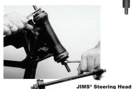
Use to install tapered steering head races and ball bearing cups into the frame on all models, straight and true. #758-725
