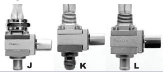
The Guzzler Fuel Valve can be used with gasoline, methanol or nitromethane. It is manufactured from aircraft aluminum and hardcoat anodized. Features include spring loaded ball detents for positive on/off positioning and stainless steel components. This valve flows 1-1/2 gallons per minute and is 1" square.
