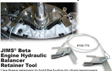
Use these retainers to hold the hydraulic chain tensioners in place when repairing all Beta engines. These are a "must have" tool for proper assembly or disassembly of the 'B' engine balancer system. #758-779
