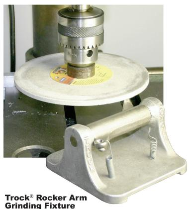
Use this fixture with a drill press mounted grinding wheel to resurface worn rocker arm pads. Badly pitted rocker arms can be welded using hard-faced rod and re-ground using this fixture. Works with Twin Cam®, Evolution®, Shovel and Sportster® rocker arms. #706-404
