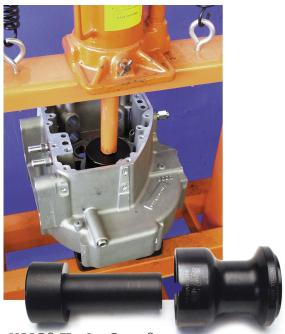
JIMS® Twin Cam® Crankshaft Bearing Tools
