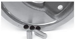
Use in special applications or repairs to add weight to flywheels when balancing. Tungsten slugs weight a little more than double that of the steel they'll be replacing. Two lengths available in 1/2" O.D.; drill the wheel, insert the slug and weld. Sold each.
