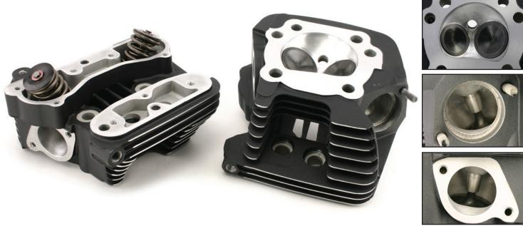
Owners of Evolution® powered Big Twins can increase their engine's output with a set of our CNC-ported EV heads! The factory casting is CNC-machined to our proven high torque, high power port shapes and the valve sizes are increased to 1.900" intake and 1.630" exhaust. Ductile iron Step-Lock guides are fitted and topped off with high quality Viton® seals and a performance spring kit. The head gasket surface is decked for flatness before final assembly. This head has substantially
