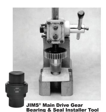
Use this tool to safely install new main drive gear inner needle bearings and seal. This tool will hold bearings and seal square to its bore, to the right depth.
