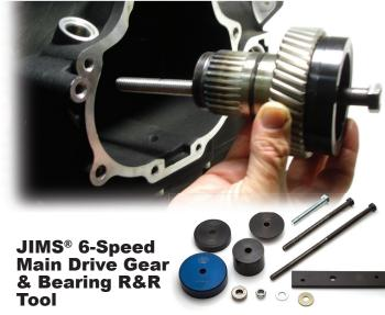
This is a complete kit for servicing the main drive gear and main bearing on the H-D<sup>®</sup> 6-speed transmission. This precision tool removes and installs both parts correctly without damaging the case. For 2006 FXD and all 2007-up Twin Cam<sup>®</sup> models. #758-900
