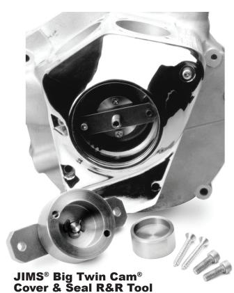
Use to remove a stubborn '70-'99 BT cam cover or remove and install the cam seal without removing the cam cover. Just mount tool in cover, screw in the two removing screws, turn center, and out comes the cam seal. The new seal is pressed in with the same tool, square and flat for a no leak fit. #758-243
