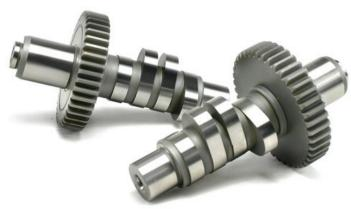
**EV 46:** Bolt-in performance cam with fast open and close ramps. Longer duration increases top-end power and torque over the EV 3. Best with increased (9+:1) compression. Power range 2600 to 6000+ RPM.
