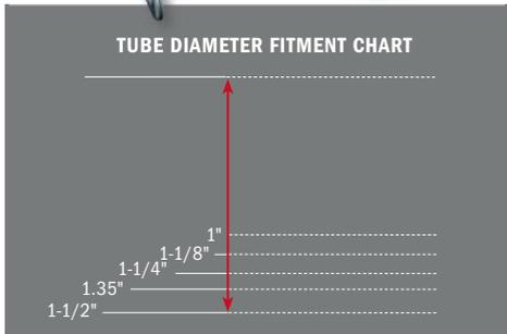
Note: To measure your tube size tighten an adjustable wrench around the tube. Remove the wrench & measure the opening. Mounting Cruise Pegs off frame tubes requires 1-1/2" of straight unobstructed tubing for clamping at equal height on both sides & approximately 3/8" of clearance around tube.
