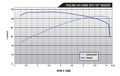
2013 Twin Cam BAGGER 107" engine. FEULING® 543 Grind camchest kit Forged 10.5:1 Compression Pistons. Stock Cylinder Heads. Bassani B4 2>1 Exhaust Big Sucker Intake.
