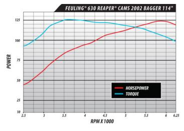
2002 Twin Cam BAGGER 114" Revolution Big Bore Kit. FEULING® Race Series 630 grind camchest kit. Conversion Camshafts.
